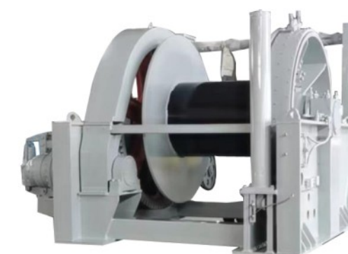
Electric towing winch Capacity: 5t~100t Rope length: 1000m Rope speed: 9~12m/min
